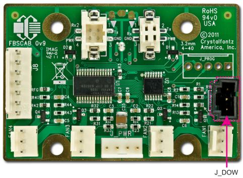
Figure 8. Location of Connection for Temperature Sensors (J\_DOW)
